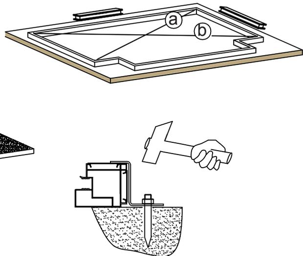
Stahlanker in Beton
